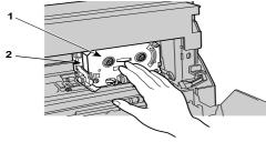
1. If an ink cartridge (1) is on the carriage (2), press on the middle of the cartridge, as shown below, to ensure it is properly seated. Also, check that the cartridges in the holders are correctly installed.
